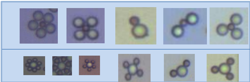
Figure 1: Ring formations after application of small acoustic field. In the case of low levels of ferrofluid, R1, R2, R3, R4 and R5 ring types are created. When the levels of ferrofluid concentration is higher, their inverse are obtained as well as R6* and R7*, where * denotes inverse configuration.
